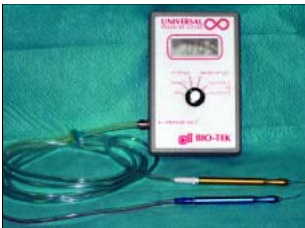
Figure 1. The authors connected the Universal Pressure Meter to the irrigation terminal.
